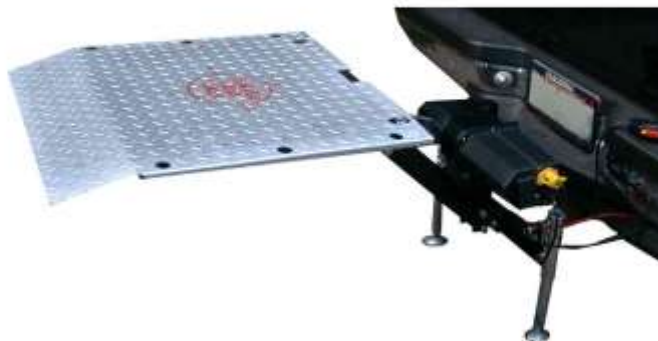
THE HITCH LIFT IN THE UP POSITION (Tailgate up for clarity.)
